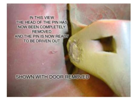
7. An alternate method of removing the upper hinge pins is to drill the head off as you would with any rivet. THIS METHOD IS RECOMMENDED TO BE USED BY PROFESSIONALS. If not done properly, damage could occur. The process is provided in the pictures below.
