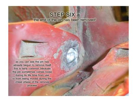
8. While maintaining a steady grip on the door, tap out the old hinge pins. Move the door slightly away from its normal position and tap out the old bushings.
